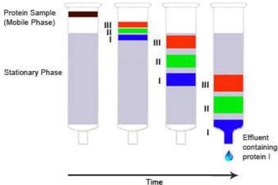
**Fig:- Chromatography Separation Technique**
