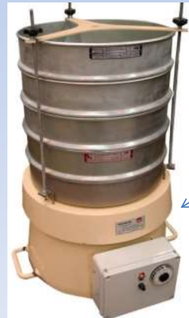
Sieve trays were put on a stack (shaker)
