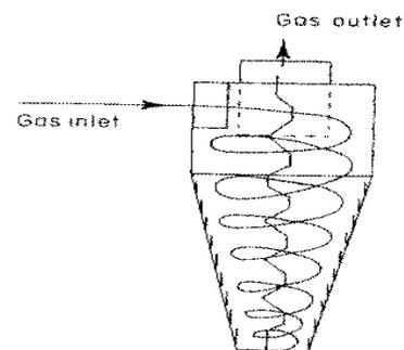
Figure 8.4 Gas flow in a gas cyclone.
