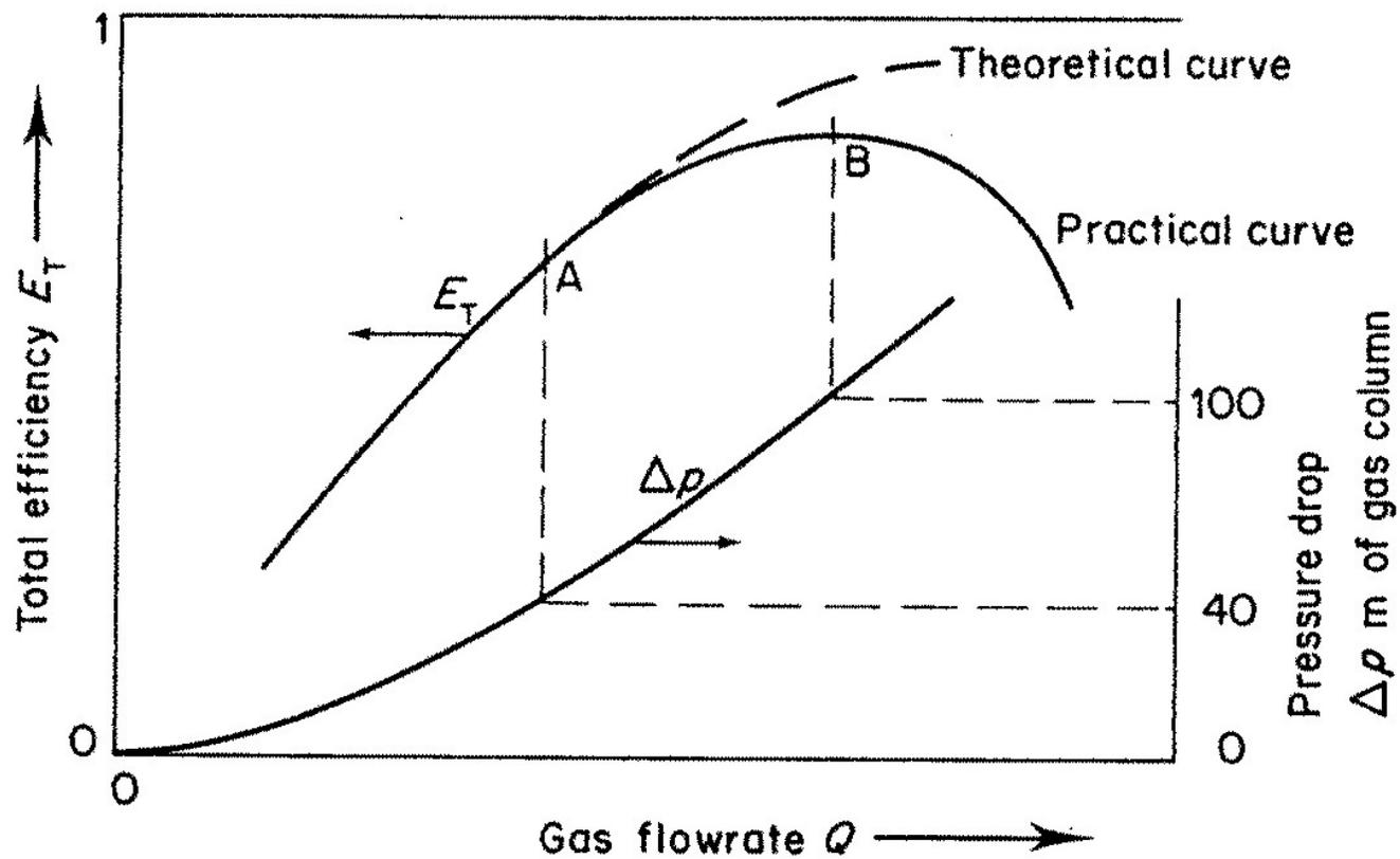
Fig. 8.6 Typical operational characteristics of gas cyclones
