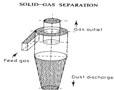
Figure 8.2 Schematic diagram of a reverse-flow gas cyclone.
