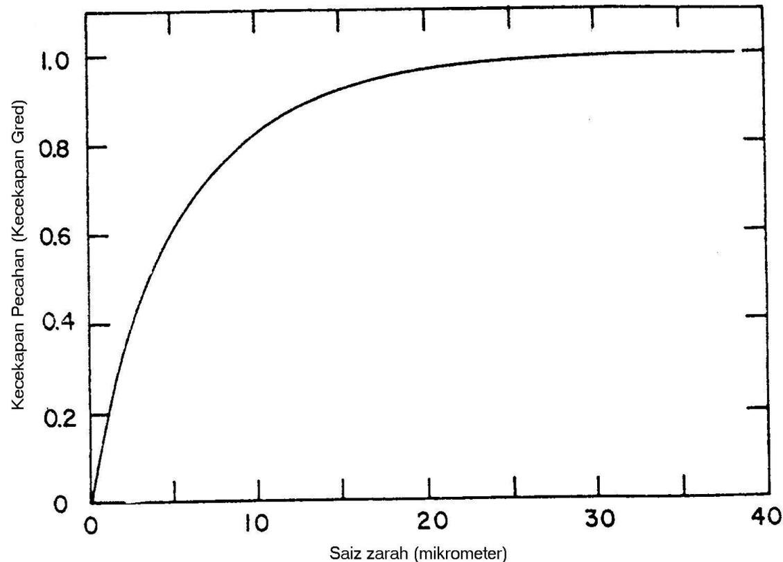
The particle size for which the grade efficiency is 50%,  $d_{50}$  is often used as a single number measurement of the efficiency of the cyclone.
